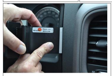
1. Clean the area where the ProClip will attach. Remove the cover from the adhesive tape on the ProClip. Place the ProClip in your hand so the ProClip label (sticker) is in an upright position.
