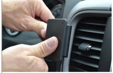
2. Rotate the ProClip to the right so the left angled edge slides under the frame that surrounds the speedometer. Then hook the right angled edge of the ProClip over the left edge of the vent frame. Press in on the angled edges to make sure the tape attaches to the dash securely.
